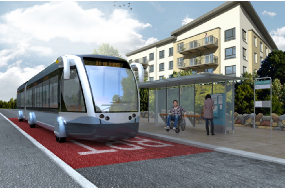
Fig. 13: Bus Rapid Transit concept - Vehicles benefit from being able to operate on segregated guided tracks as well as on roads, therefore offering greater route choice and flexibility than heavy or light rail options.
