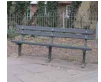
SEAT TYPE D: formed of Recycled materials, plastic slats, steel frame. Appropriate along the river walk, though should be avoided in streets and urban spaces
